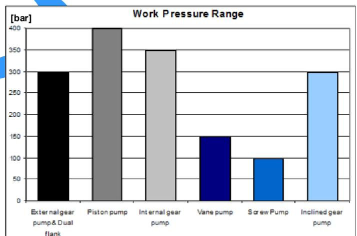
On the side: comparison between the different fields of use of different kinds of volumetric pumps.
