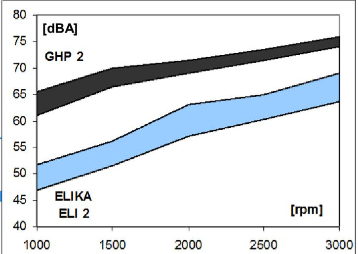
Noise pump comparison [dBA] Marzocchi GHP2 – ELIKA ELI 2, same displacement 17.8 cm<sup>3</sup>/rev, pressure from 10 to 250 bar.
