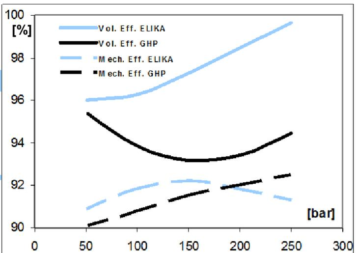
Efficiency pump comparison [%] Marzocchi GHP2 – ELIKA ELI 2, same displacement 17.8 cm<sup>3</sup>/rev, rotation speed 1500 rpm.
